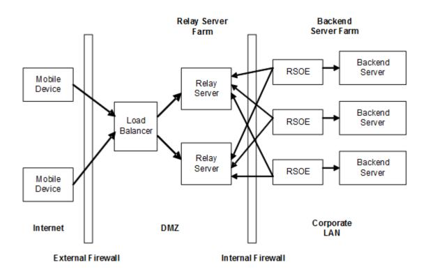
The Relay Server consists of a web server, three web extensions (an administration extension, a client extension, and a server extension), and a background process for maintaining state information (Apache only). The client extension handles client requests made from applications running on mobile devices. The server extension handles requests made by the Outbound Enabler on behalf of a backend server.
